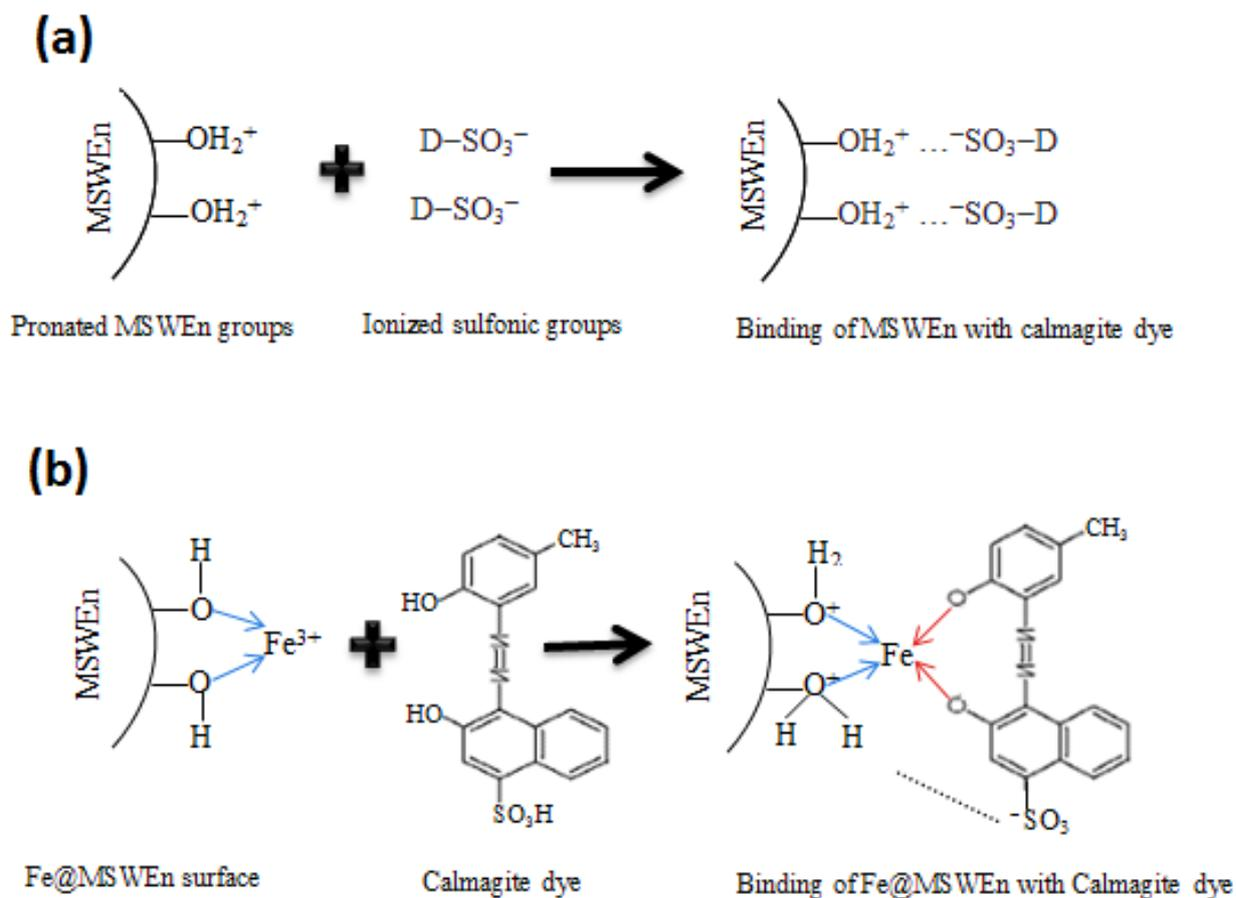
**Scheme 1:** Suggested mechanisms of: (a) the ionic interaction between MSE and Calmagite dye, (b) the ternary complex formation and ionic interaction between Fe@MSWEn and Calmagite dye
