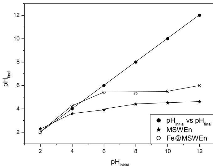
**Figure 5:** Plot for determination of point zero charge of MSWEn and Fe@MSWEn adsorbents
