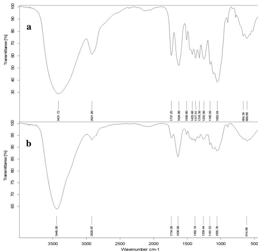
**Figure 2:** FT-IR spectra of (a) MSWEn and (b) Fe@MSWEn adsorbents
