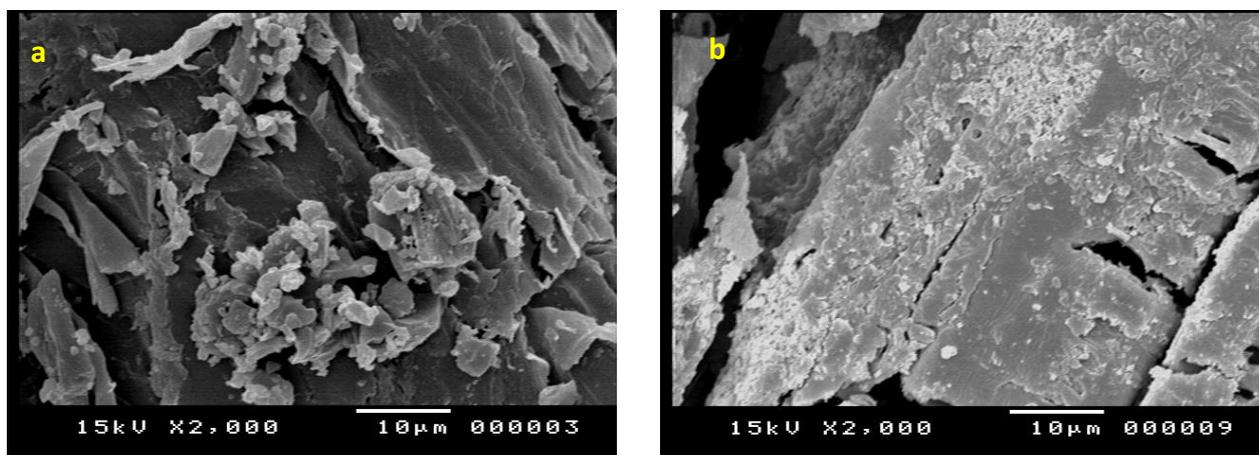
Figure 4: SEM micrographs of (a) MSWEn and (b) Fe@MSWEn adsorbents
