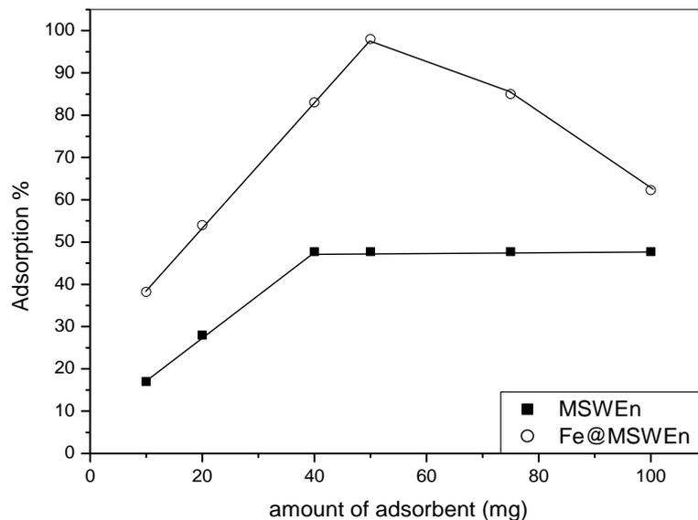
**Figure 7:** Effect of adsorbent amount on adsorption percent of MSWEn and Fe@MSWEn adsorbents
