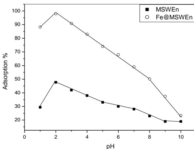
**Figure 6:** Effect of pH on adsorption percent values of MSWEn and Fe@MSWEn adsorbents
