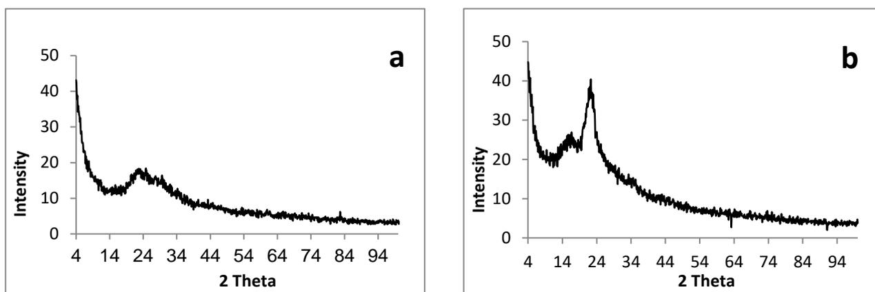
Figure 3: X-ray diffraction patterns of (a) MSWEn and (b) Fe@MSWEn adsorbents
